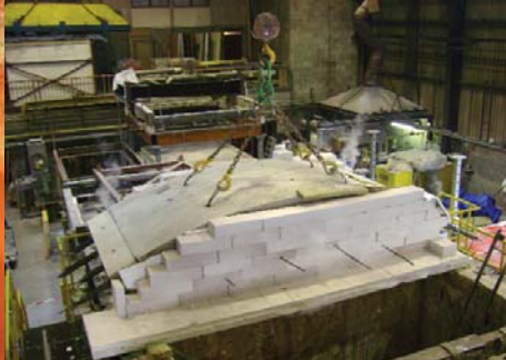
FIGURE 13: TEST SET UP FOR A FULL SIZE TUNNEL SEGMENT
