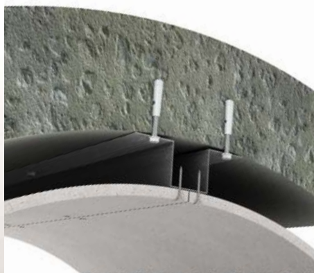
FIGURE 52: SECTION THROUGH CURVED CONCRETE SECTIONS
