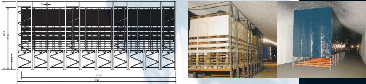
FIGURE 7: SET-UP FOR TEST #2 (WOOD PALLET AND PUR MATTRESSES)
